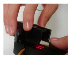
3) Slightly press the optical fiber into the slot of the shade cover and put it on the palm, then we can get the accurate measurement result.
