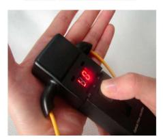
4) Once testing is complete, remove the shade cover on the OFI.
