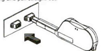
When pushing, do not apply excessive force or apply force in a different direction than indicated by the arrow. Cleaning an Optical Connector Plug
