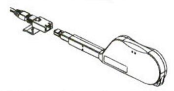
③ Insert the main body straight in to the Optical Connector Plug. When you hear the click sound, the cleaning is completed. Stop pushing and remove straight out.
